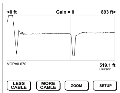
Figure 3 – Trace of a Short – Negative Reflection – Conductors Moving Closer Together
