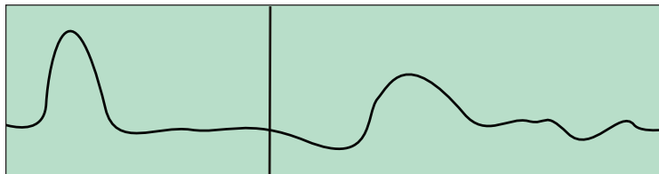
Figure 6: Water in the Cable (example)
