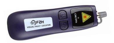
The VLS8 series visible laser source is the first tool to add to any fibre optic tool bag. Nothing can find a fibre fault that is close by better than a visible light source. The VLS8, with its small size and long battery life, make this the ideal visible source to fault find patch cords, pigtails and connectors when an OTDR is unable to find a fault that is too close to the source.
