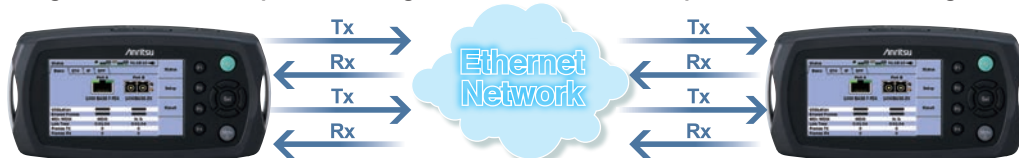
Bidirectional performance test with End-to-End RFC 2544, Two ports simultaneous testing for multiple ports installation.
